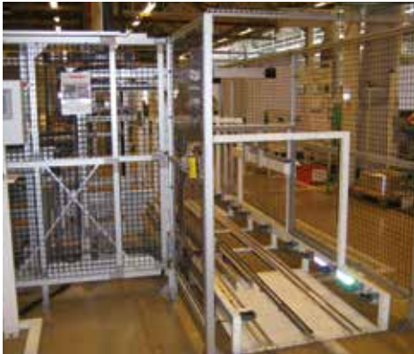
Quick-Guard Standard assembled with mesh.
