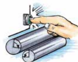
Shaft only turns a small amount each time the PB is pressed.
