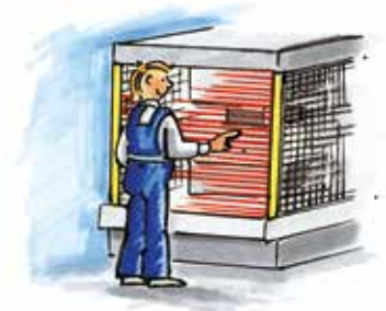
Resolution for finger ( \leq 14 mm) gives C = 0
