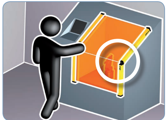
The resolution is maintained (up to 40 mm) in the junction between the 2 protected areas
